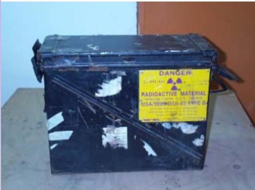
*FIG. 9. Overpack for the source container.*
