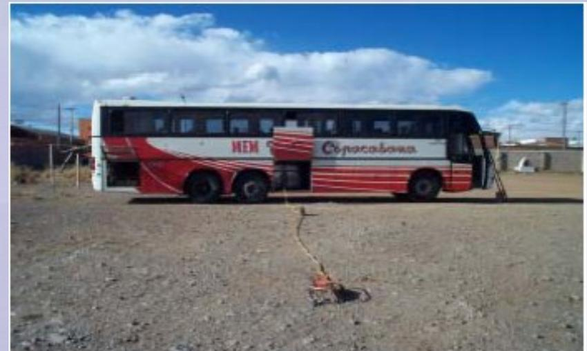
FIG. 18. Reconstruction by the IAEA of the circumstances of the accident. In the foreground is the radiography equipment with its guide tube unwound up to the cargo compartment of the bus.
