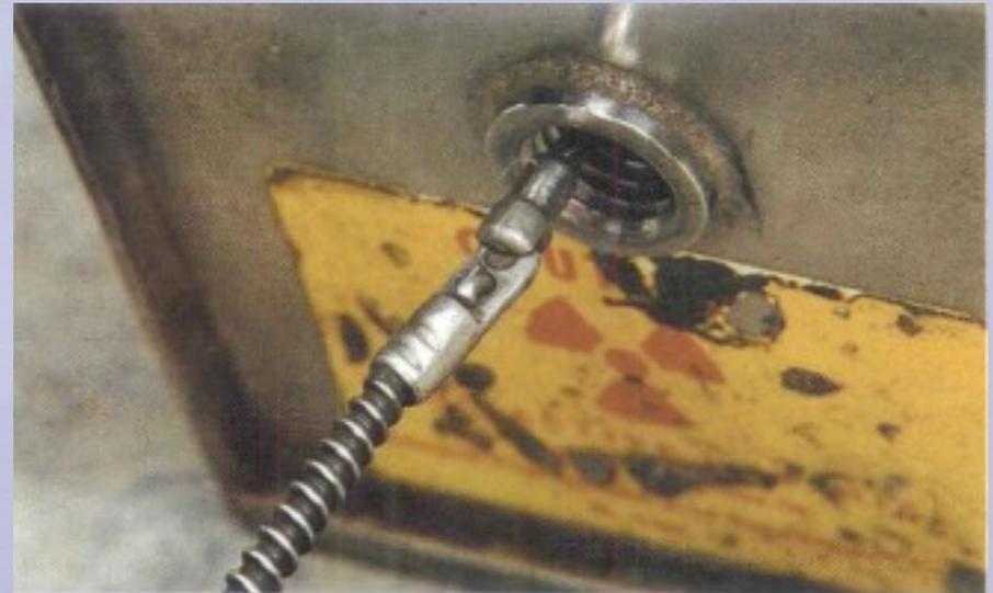
*Photo 2. Source pigtail connected to drive cable.*
