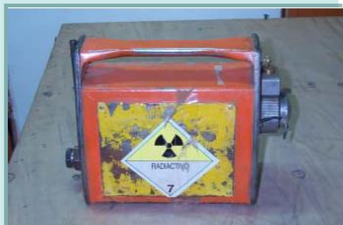
FIG. 2. Industrial radiography container involved in the accident in Cochabamba.
