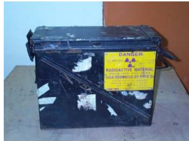
FIG. 9. Overpack for the source container.
