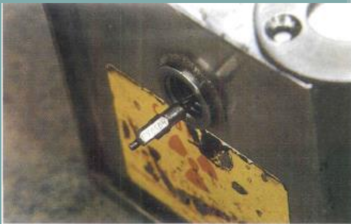
Photo 1. Source pigtail ready for connecting to drive cable.
